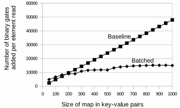
Figure 15. Per-element cost of performing  $n$  read operations on an array of  $n$  elements. Baseline uses a simple multiplexer, while the “batched” circuit uses an associative map. All maps are integer-to-integer maps, values being 16-bit integers and keys  $(\log_2 n)$ -bit integers.
