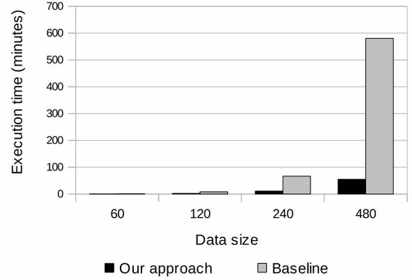
Figure 20. Execution time for DBSCAN clustering protocol over garbled circuits. Data size is in number of data points, where each data point is simply an  $(x, y)$  pair of two 16-bit integers, and the distance metric used is Manhattan distance.
