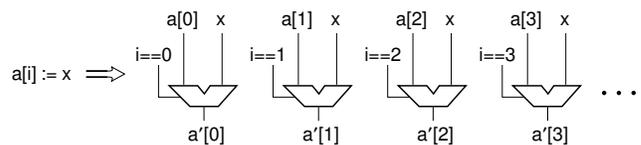
Figure 1. A single array access requiring  $n$  multiplexers.
